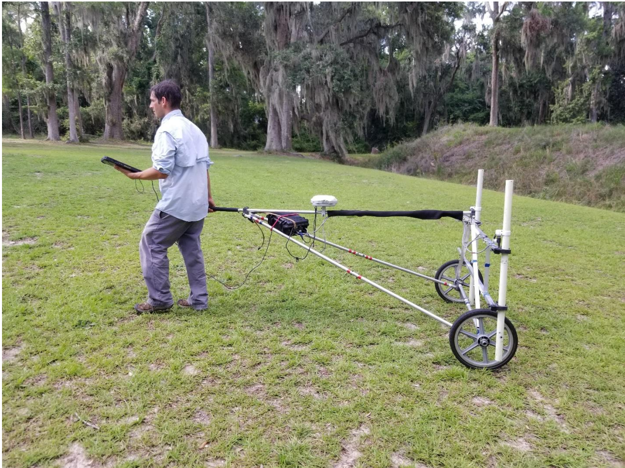
Figure 2. Photograph of magnetometer and GPS setup.
